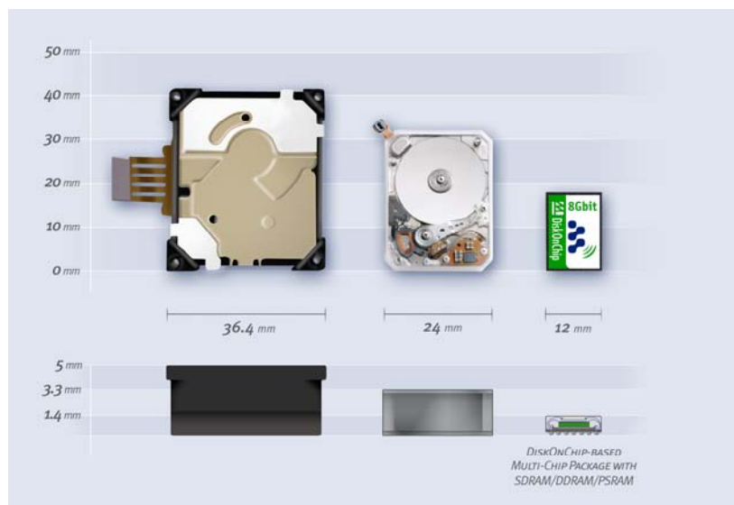
Figure 1: Popular Micro Drive vs DiskOnChip Dimensions
